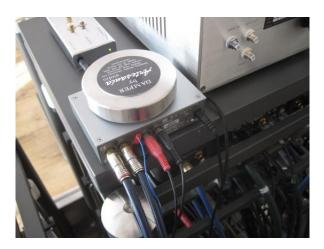
The Schiit Mani MM/MC phono preamp at only 160 euro is excellent value for sure. The Mani was used at the gain setting that best matched the comparison unit and at its 47k ohm setting for MM
